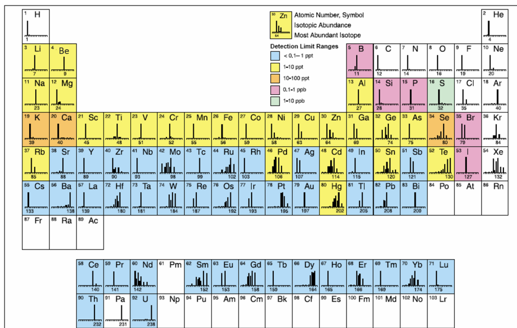
Figure 10: The different ICP-MS spectra and limits of detections for the elements. Elements in the white boxes cannot be measured in this way.
