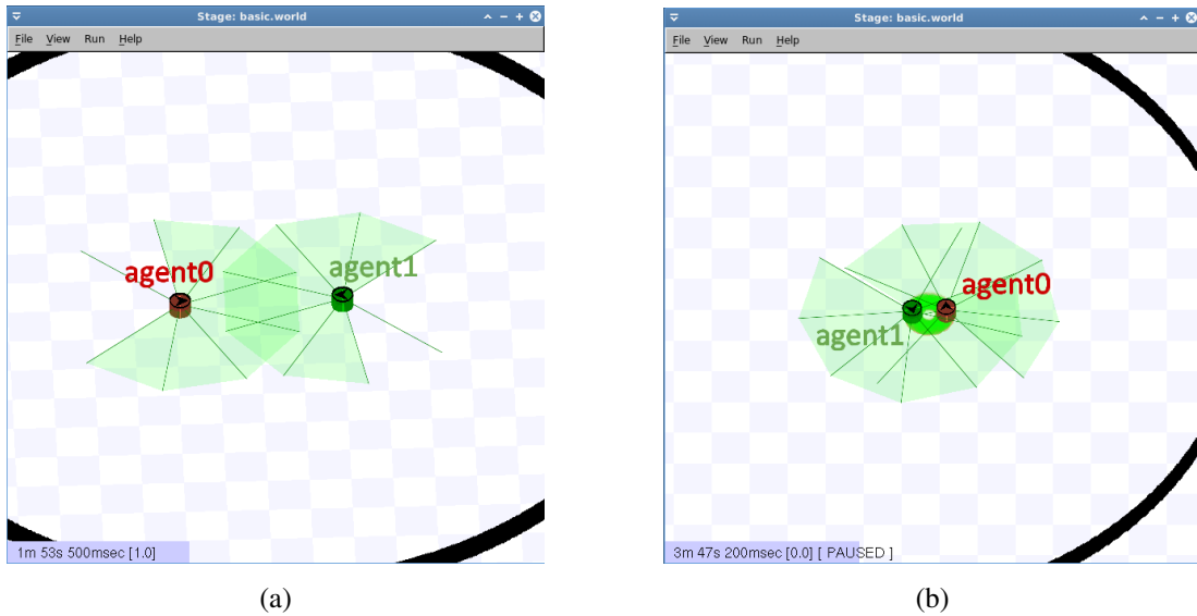
Figure 4.9: (a): Starting positions for agent0 (expert) and agent1 (learner) in the Stage simulator. The agents are facing each other but are not in sensory range. (b): The two agents successfully “dancing”; this is detected and rewarded.
