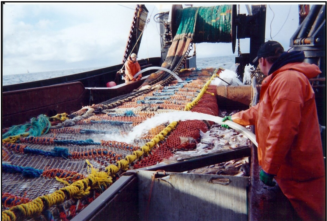
Spilling the fish out of the cod end and into a fish hold.
