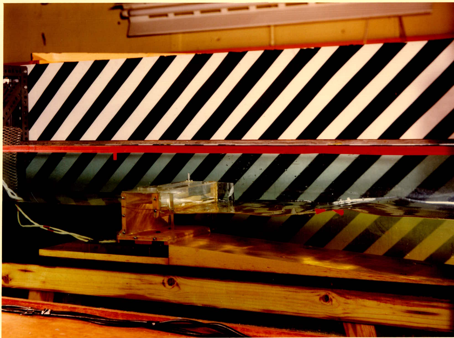
MODEL BREAKWATER DEVICE UNDERGOING TESTS IN THE NEL TWO DIMENSIONAL WAVE TANK
