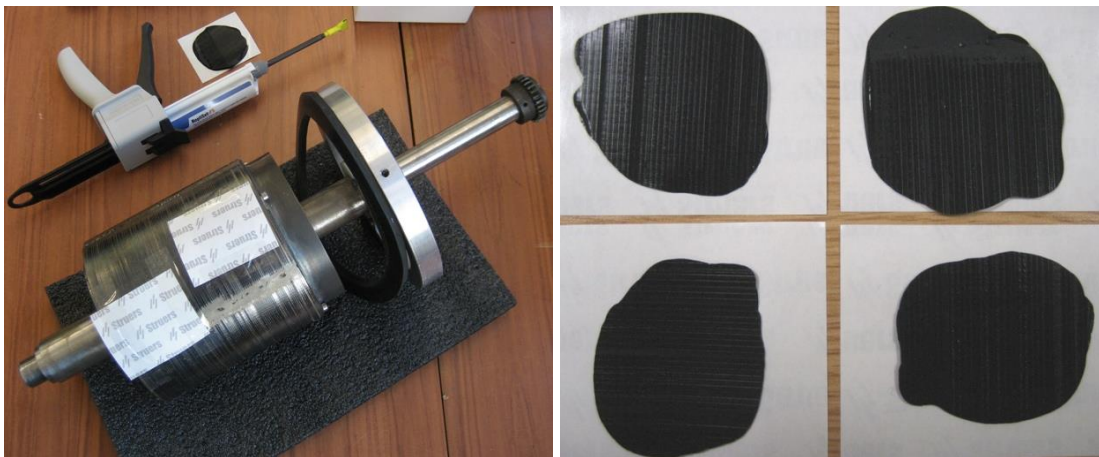
Figure 7.8: Replicating the surface condition of rotor laminations using RepliSet-F5
