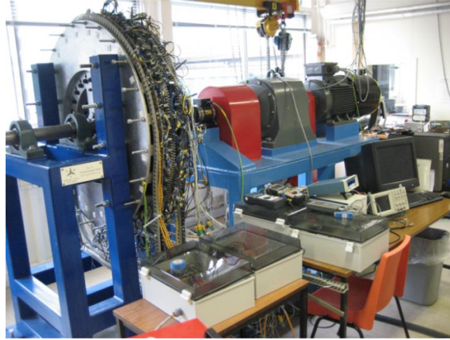
Figure 4.2: 25 kW AFPM prototype at the experimental test facility
