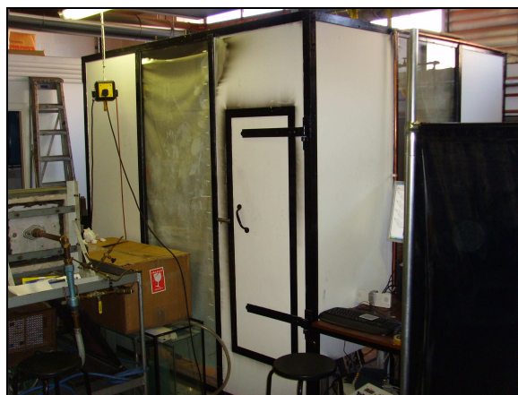
Figure 4.20 – The compartment in which the experiment was housed was filled as extensively as possible with particle seeding.
