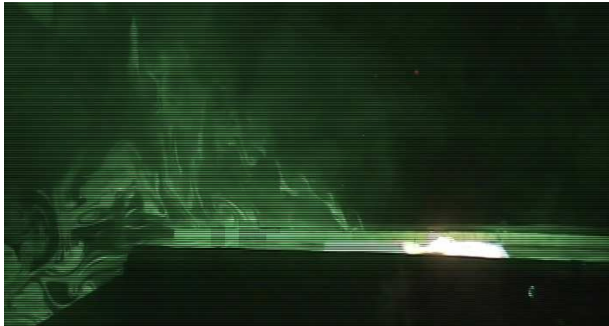
Figure 6.17 – The images show the highlighted patterns of the seeding particles by the laser during measurements by the PIV system.
