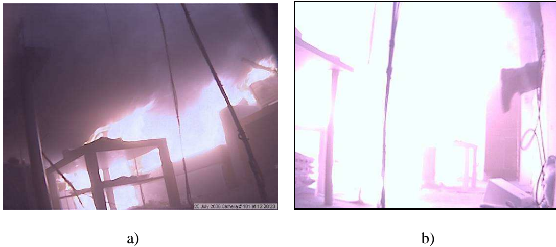
Figure 1.3 - Images from a) Test One and b) Test Two show the tests at almost identical times post ignition and pre-flashover, taken from the same locations with respect to the experiments. Even though both scenarios are in the early stages of flashover, the conditions appear very different when just the information afforded by the images is taken into account.
