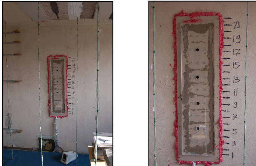
Figure 4.4 – The image shows the sample mounted in the compartment fire experiment of Dalmarnock Fire Test One.
