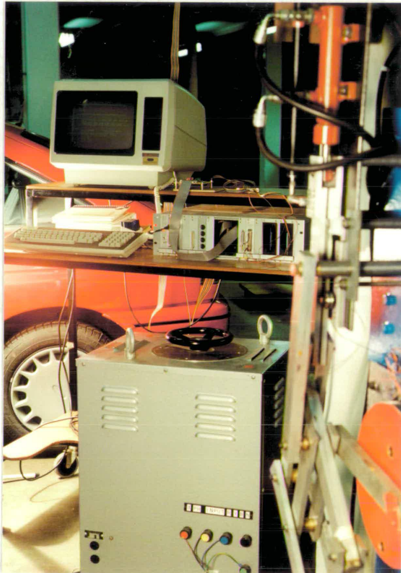
Photograph A2.3 The leg mechanism driven by computer control. The 3-phase variac supplying power to the test rig and the straight line potentiometer in parallel to the hydraulic ram can also be seen.
