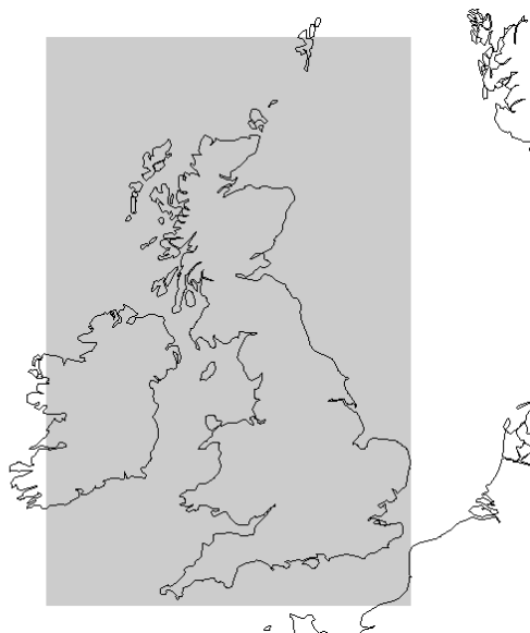
Figure 6-1. Model domain used for the comparison of FRAME and CMAQ results. The domain is in British National Grid projection. The resolution is 5 x 5 km 2 .
