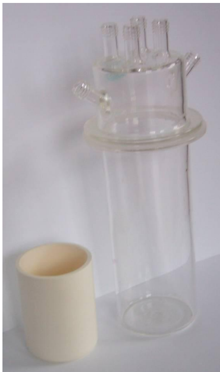
Figure 8-2: The quartz cell with alumina crucible
