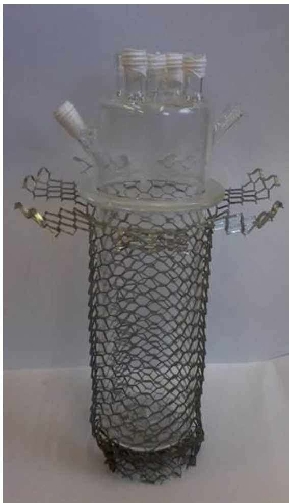
Figure 8-13: Metal cage designed to act as a pseudo-faraday cage.
