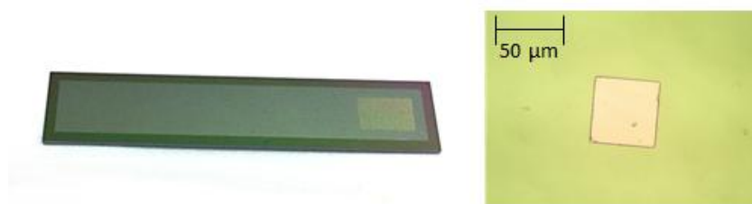
Figure 5-1: Square microelectrode device with contact pad. Microscope image shows a 50 \mu\text{m} edge microelectrode.
