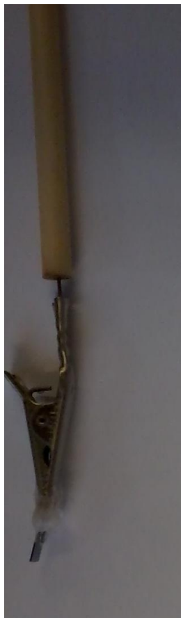
Figure 8-9: The microelectrode device and crocodile clip sealed in ceramic gum to prevent loss of connection.
