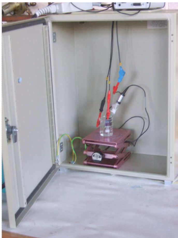
Figure 3-9: The experimental set up of the three electrode system including microelectrode in a Faraday cage for room temperature aqueous characterisation.
