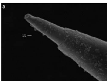
Figure 1-2: Tungsten microelectrode tip plated in platinum and characterised by SEM 42
