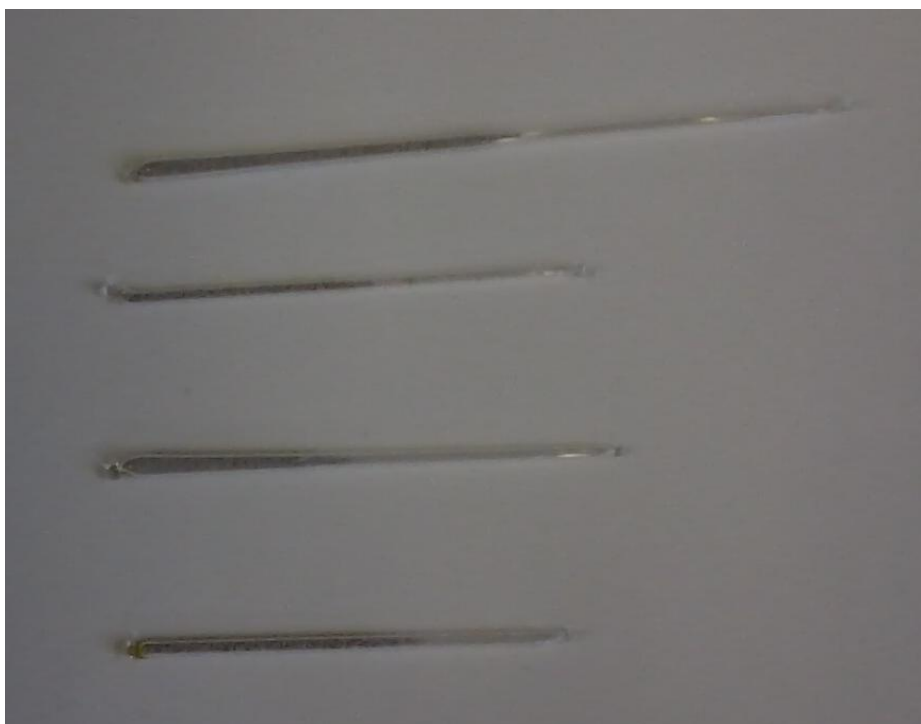
Figure 8-6: The capsules of silver chloride produced from melting point tubes that are designed to break on entry to the molten salt to release the redox active material.
