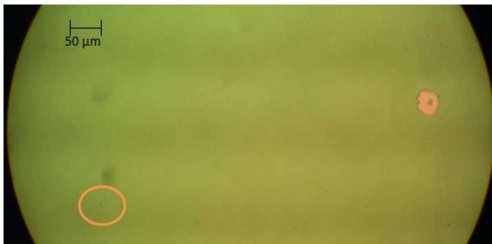
Figure 5-10: Image of the 10 \mu\text{m} length square microelectrode (circled bottom left) relative to the breakage in the passivation layer.
