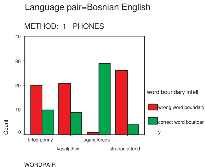
Figure 4.5: Word boundary recognition rate for Bosnian-English word pairs synthesized by PHONE method
