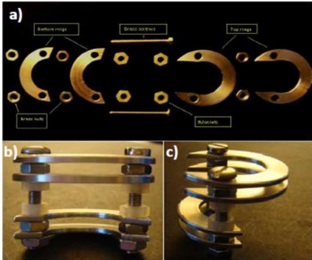
Figure 2.7 The External fixator device used in the generation and fixation of non-unions in Rats: (a) layout prior to assembly (b) Coronal view and (c) lateral view of external fixator
