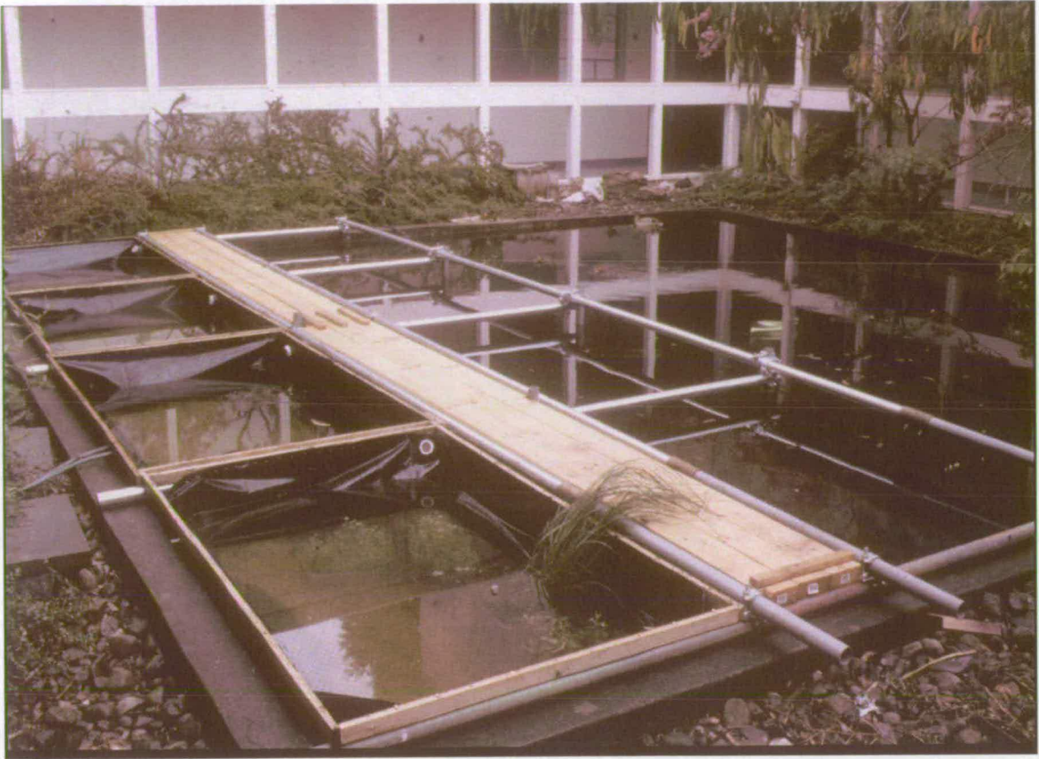
Figure 6.2. Photograph of replicate ponds. Strips of pond liner were stapled to an upper and lower wooden frame to form identical rectangular ponds. These were then sunk into a pre-existing concrete walled pond and the upper wooden frames were supported by a scaffolding framework (see Appendix IV).
