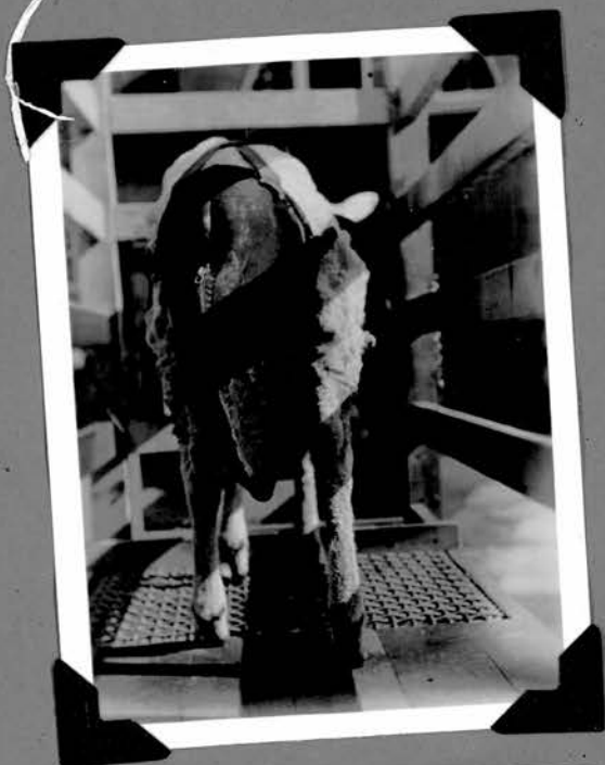
Plate XI. Metabolic bag with "zipp" fasteners.
