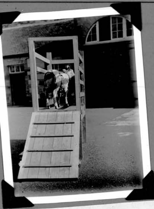
Plate X. The arrangements in sheep metabolic cage with the door lowered for emptying the bag.
