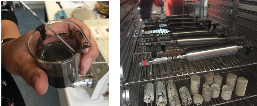
FIGURE 15 – SHALE AND FLUID MIXTURE READY FOR FILLING BATCH REACTOR (LEFT) AND FILLED AND PRESSURISED BATCH REACTORS IN THE OVEN FOR HEATING (RIGHT).
