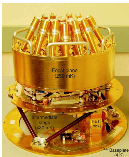
Figure 3.8: The QUaD receiver, including the orthogonal PSB feeds which are installed on the focal plane at very low temperatures. (Figure from QUaD collaboration: J. Hinderks et al., 2008)
