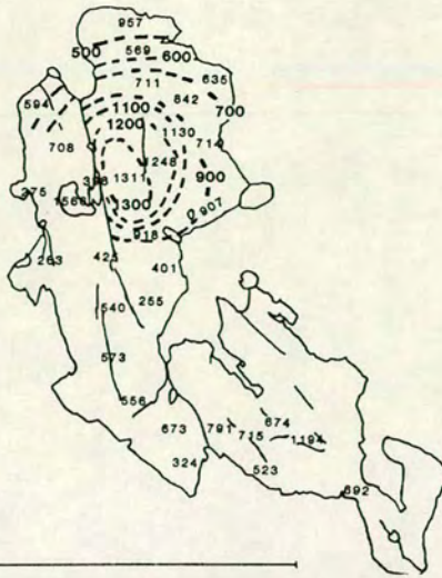
FIG. 7.12(a). Chrontour map of altered hornblende grain E16G1 as shown in Plate 55 and Fig.7.11. Note that where secondary amphibole has developed the ages are generally much lower than those of the unaltered hornblende.
