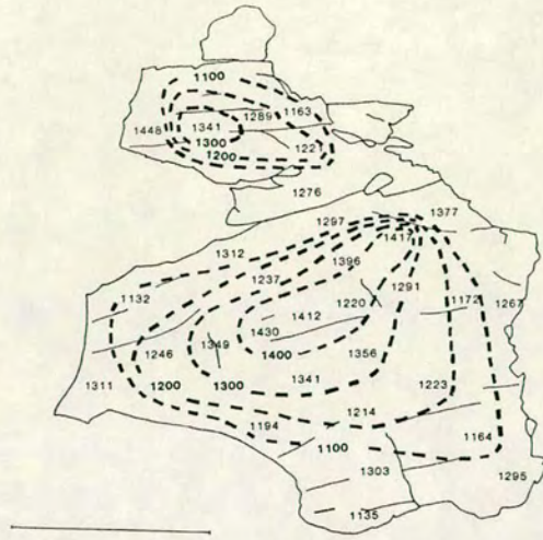
FIG. 7.8(a). Chrontour map of hornblende grain E52G2 as shown in Fig 7.7. Dates are in millions of years.
