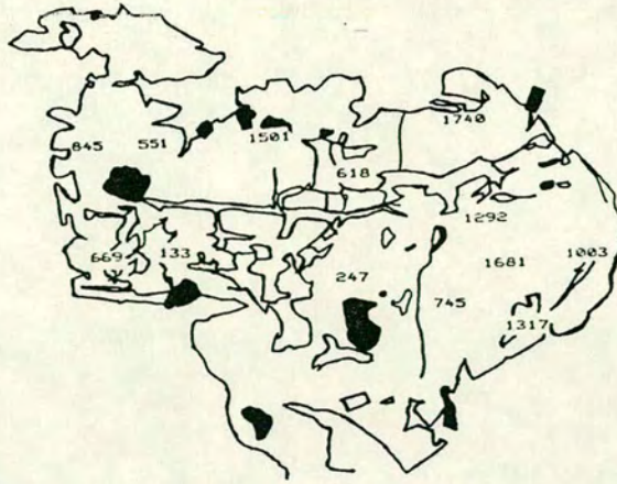
FIG. 7.16(a). Sketch showing the age variations within hornblende grain E15G2 as shown in Fig 7.15. Dates are in millions of years.
