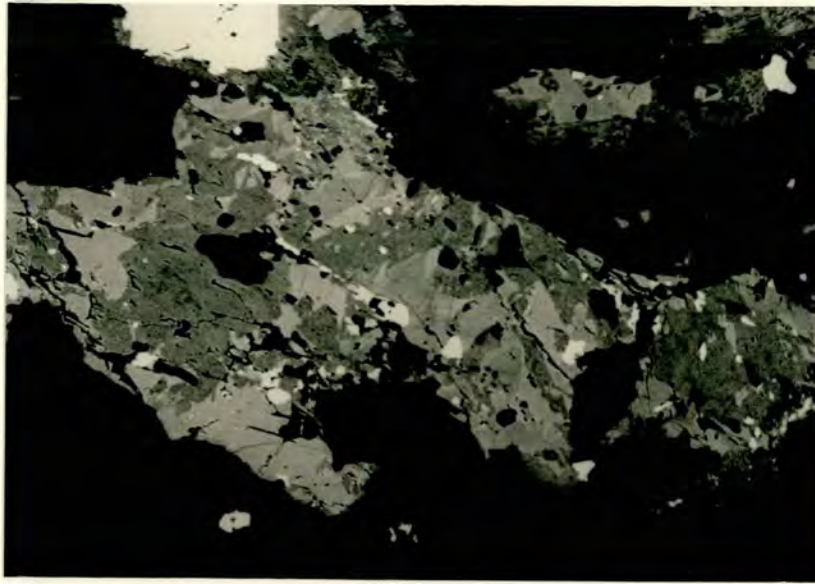
FIG. 7.13(a). B.S.E. image of altered hornblende grain 1 from rock E15 (E15G1). Scale bar: 400 \mu m.
