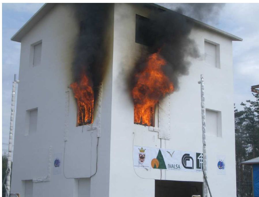
Figure 2.11: External flaming from encapsulated CLT compartment (from [153]).
