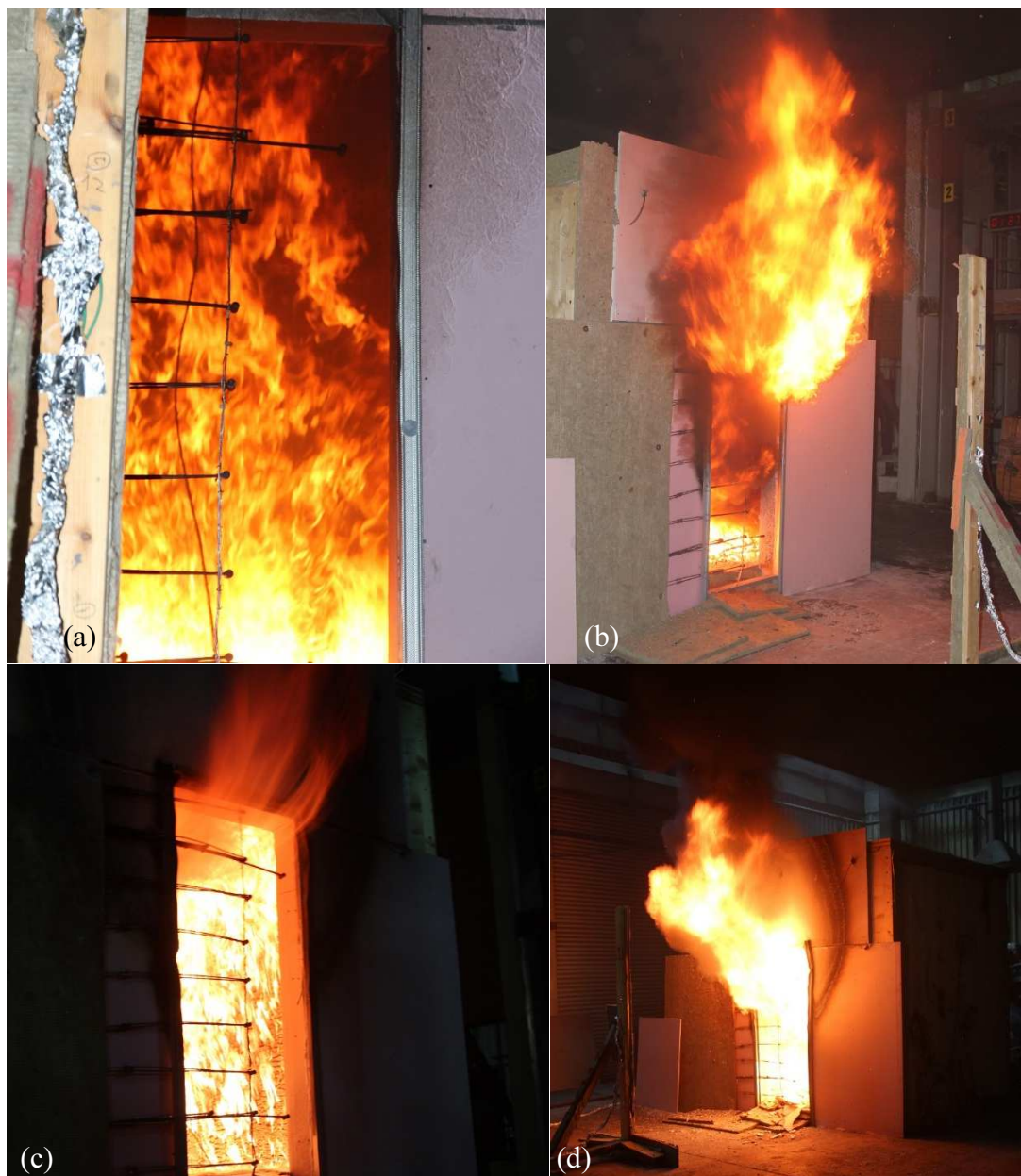
Figure 4.10: Experiment \alpha -2 (a) 5 minutes after ignition, showing flaming on back wall prior to flashover, (b) 9 minutes after ignition, showing peak external flaming, (c) 30 minutes after ignition, showing reduced external flaming and flaming on side wall, (d) 56 minutes after ignition, showing return to peak external flaming.
