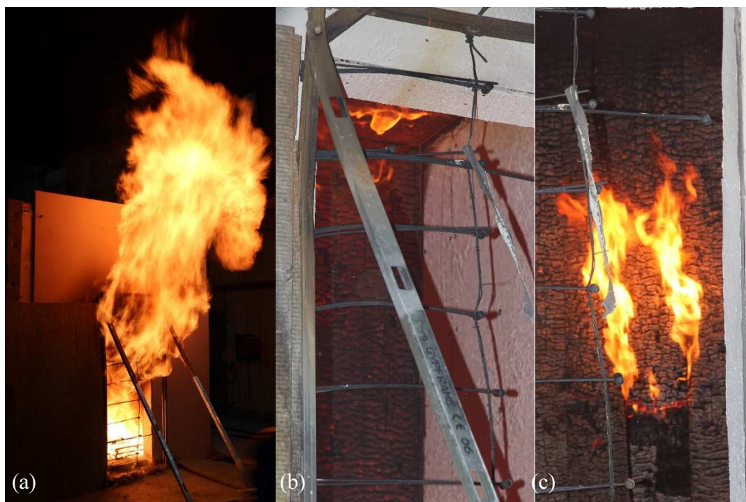
Figure 4.11: Experiment \beta -1 (a) 9 minutes after ignition, showing peak burning, (b) 21 minutes after ignition, showing cessation of external flaming and tendency towards auto-extinction, (c) 31 minutes after ignition showing localized delamination resulting in localized surface flaming.
