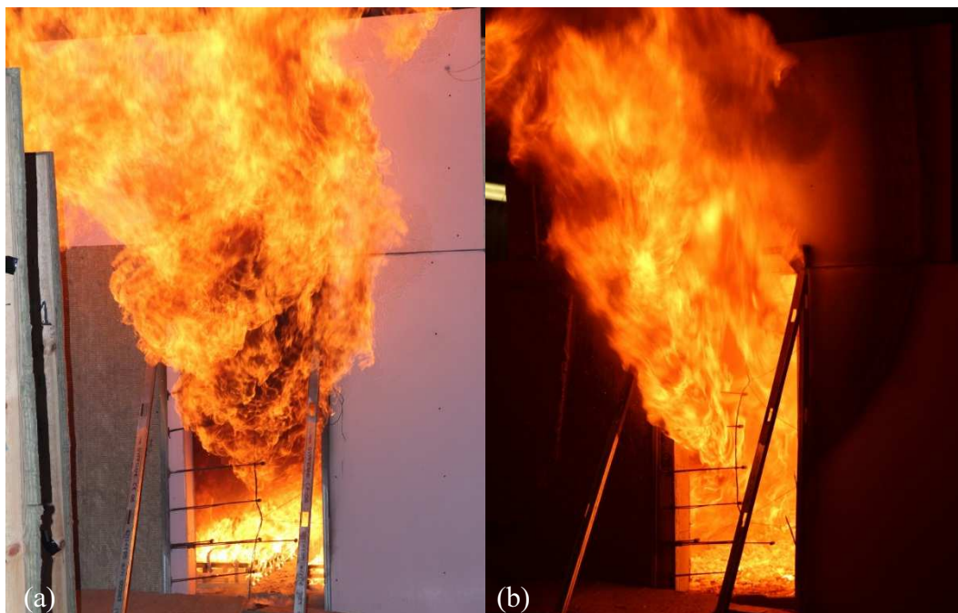
Figure 4.13: Experiment \gamma -1 (a) 6 minutes after ignition, showing peak burning, (b) 35 minutes after ignition, showing quasi-steady burning.
