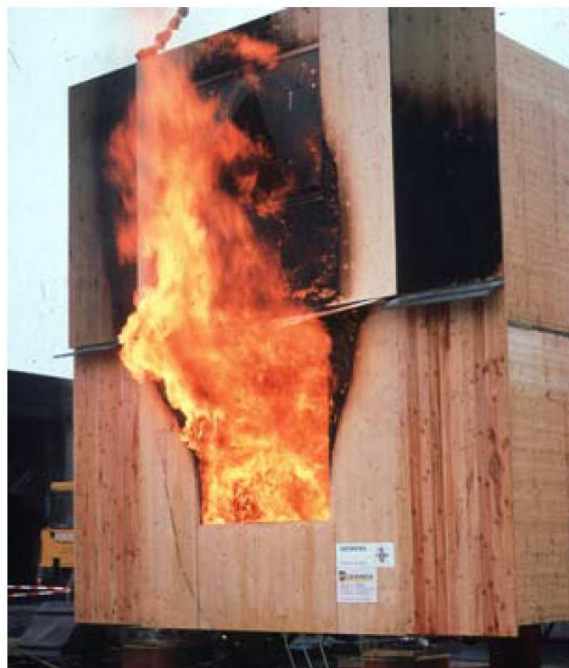
Figure 2.10: External flaming from modular timber hotel with flammable internal linings (from [152]).
