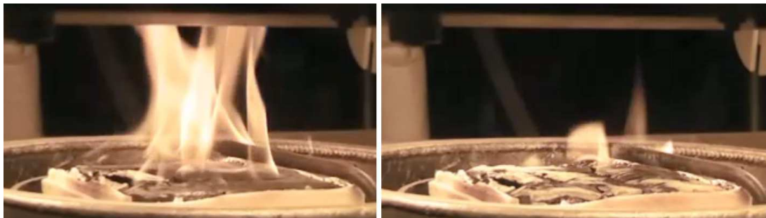
Figure 3.4: Initial (left) and residual (right) flaming during experiment IM-14-1.
