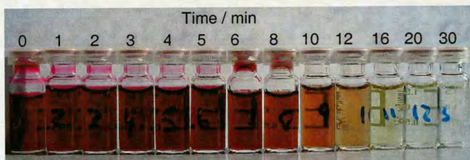
Figure 5.37 Illustration of the changes in colour which occur on ozonolysis
