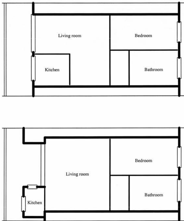
Figure 10.2: Proposed designs for single-bedroom deck-access flats (a) with a rectangular floorplan (b) with one flat overlapping the next
