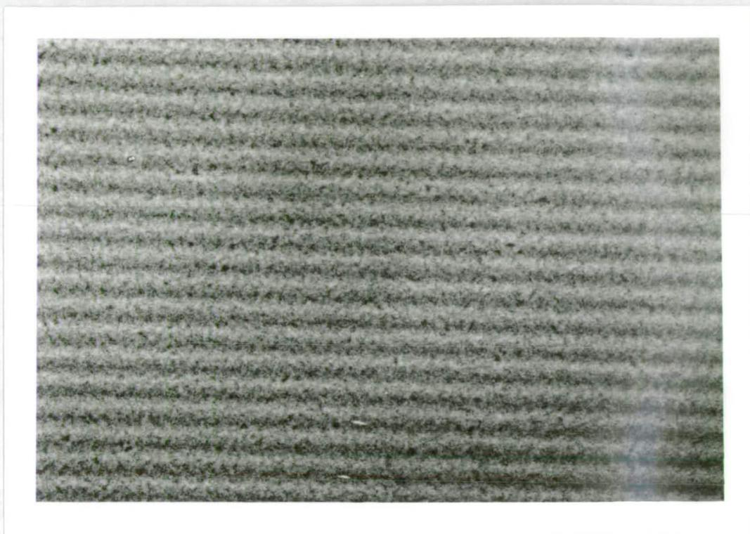
Figure 7.11. Phase-contrast micrograph of a grating made at 383 K (110 °C) using white light exposure through a mask of 12  $\mu\text{m}$  period. The  $\text{As}_{40}\text{S}_{60}$  and Ag film thicknesses are 600 and 67 nm respectively.
