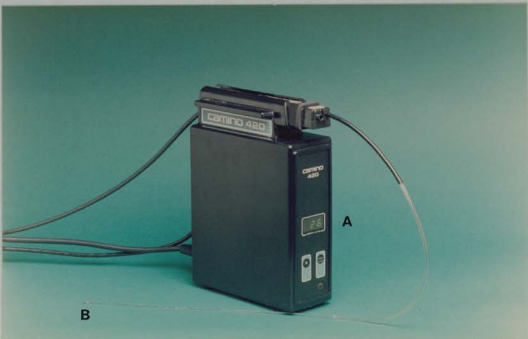
Figure 9: Camino Catheter-Tip Transducer System. A, Camino 420XP high frequency research monitor; B, Camino catheter-tip ICP transducer.
