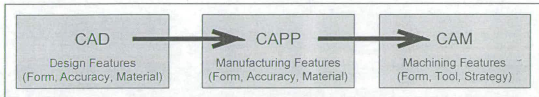
Figure 1.9 CAD-CAPP-CAM Process Chain
