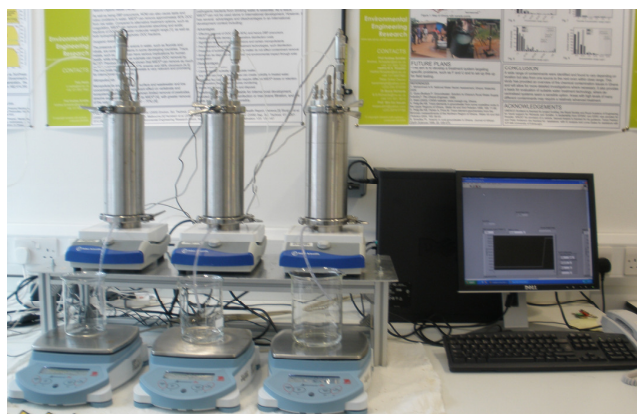
Figure 4-4 Stirred cell apparatus used for filtration experiments
