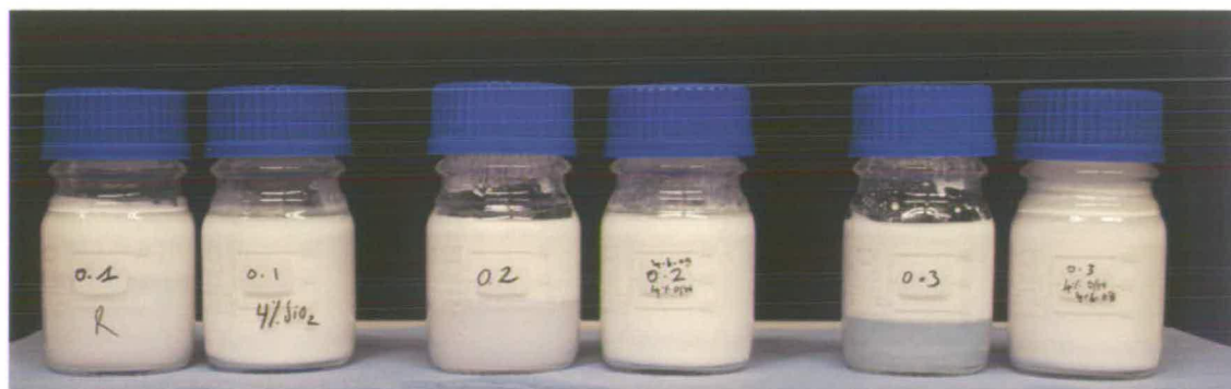
Figure 4.18: A picture of the emulsions C1, D1, C2, D2, C3 and D3 (from left to right) displaying the effect of O/W volume fraction and silica particles concentration on the emulsion stability.
