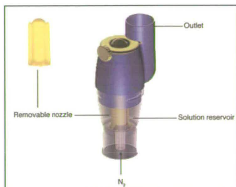
Figure 3.2: Representation of the Andy flow nebuliser.
