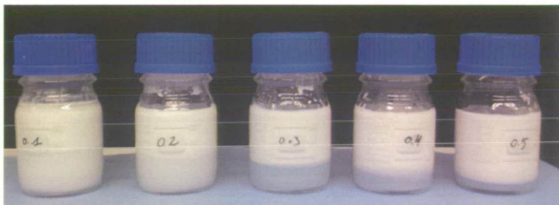
Figure 4.17: A picture of the emulsions C1 to C5 displaying the effect of volume fraction on the emulsion stability. Left to right, the O/W volume fraction are 10%, 20%, 30%, 40% and 50%.
