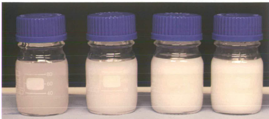
Figure 4.21: A picture of the emulsions E1, E2, E3 and E4 (left to right displaying the effect of O/W volume fraction).
