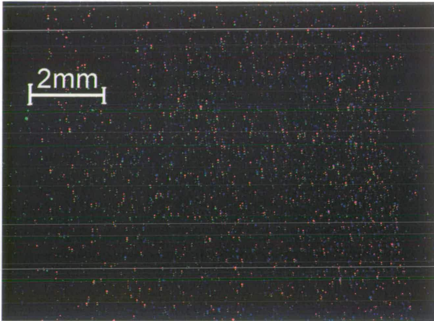
Figure 5.9: A second example of a multi-constituent flow. The RGB image shown was produced by illumination with 532 nm and 355 nm laser light sheets and a pulse separation of 50 \mu s.
