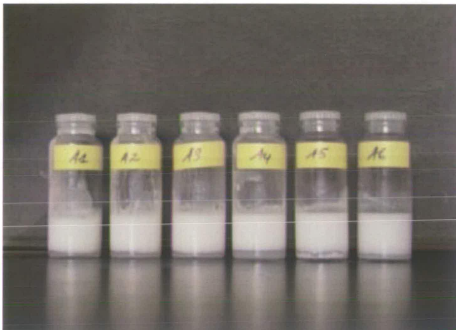
Figure 4.9: A picture of the emulsions A1 to A6 displaying the effect of volume fraction on the emulsion stability.
