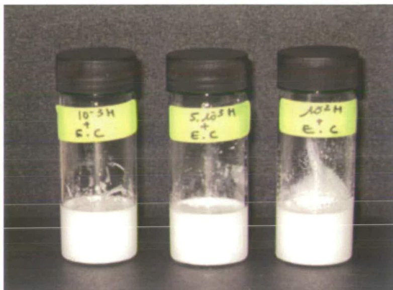
Figure 4.20: A picture of the formulation D1 emulsions at different doping level of Bis-MSB in o-xylene phase. Left to right: 10^{-3} , 5 \times 10^{-3} and 10^{-2} M.
