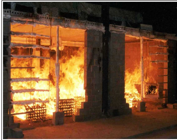
Figure 8. BRE large compartment fire test
