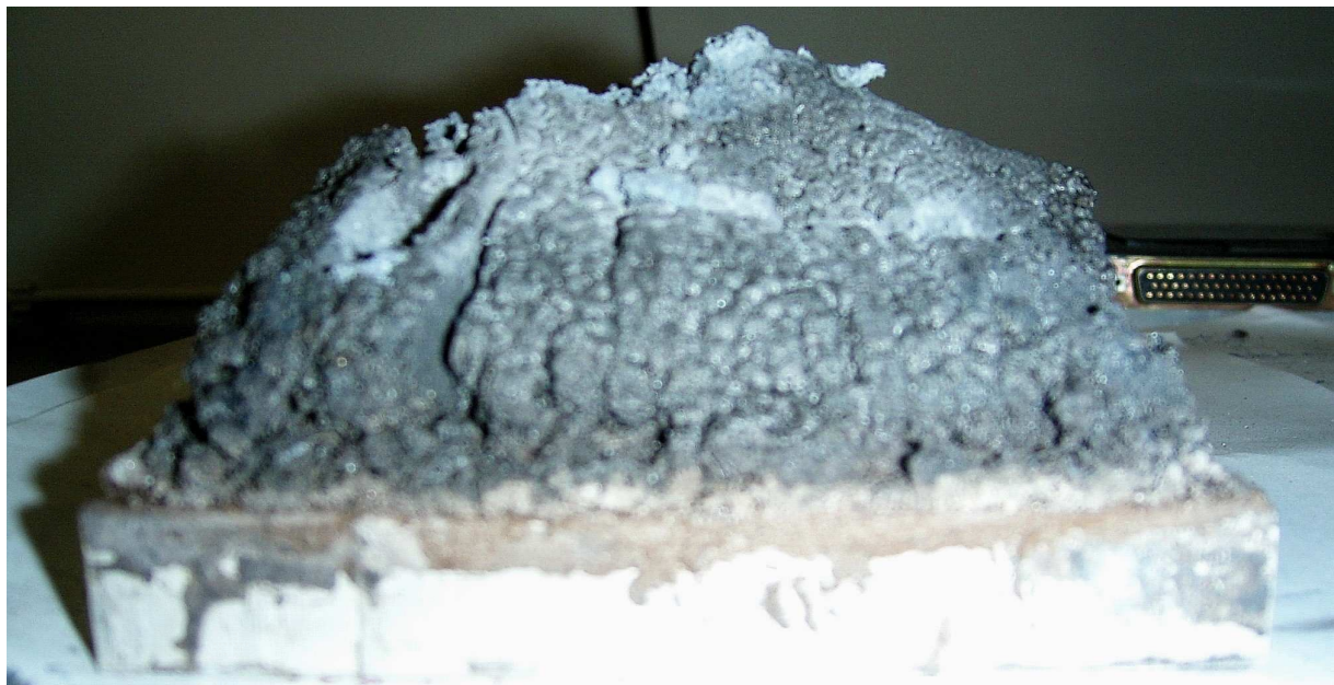
Figure 3. Photograph illustrating final condition of intumescent in test 5 (2mm, 60kW/m 2 )
