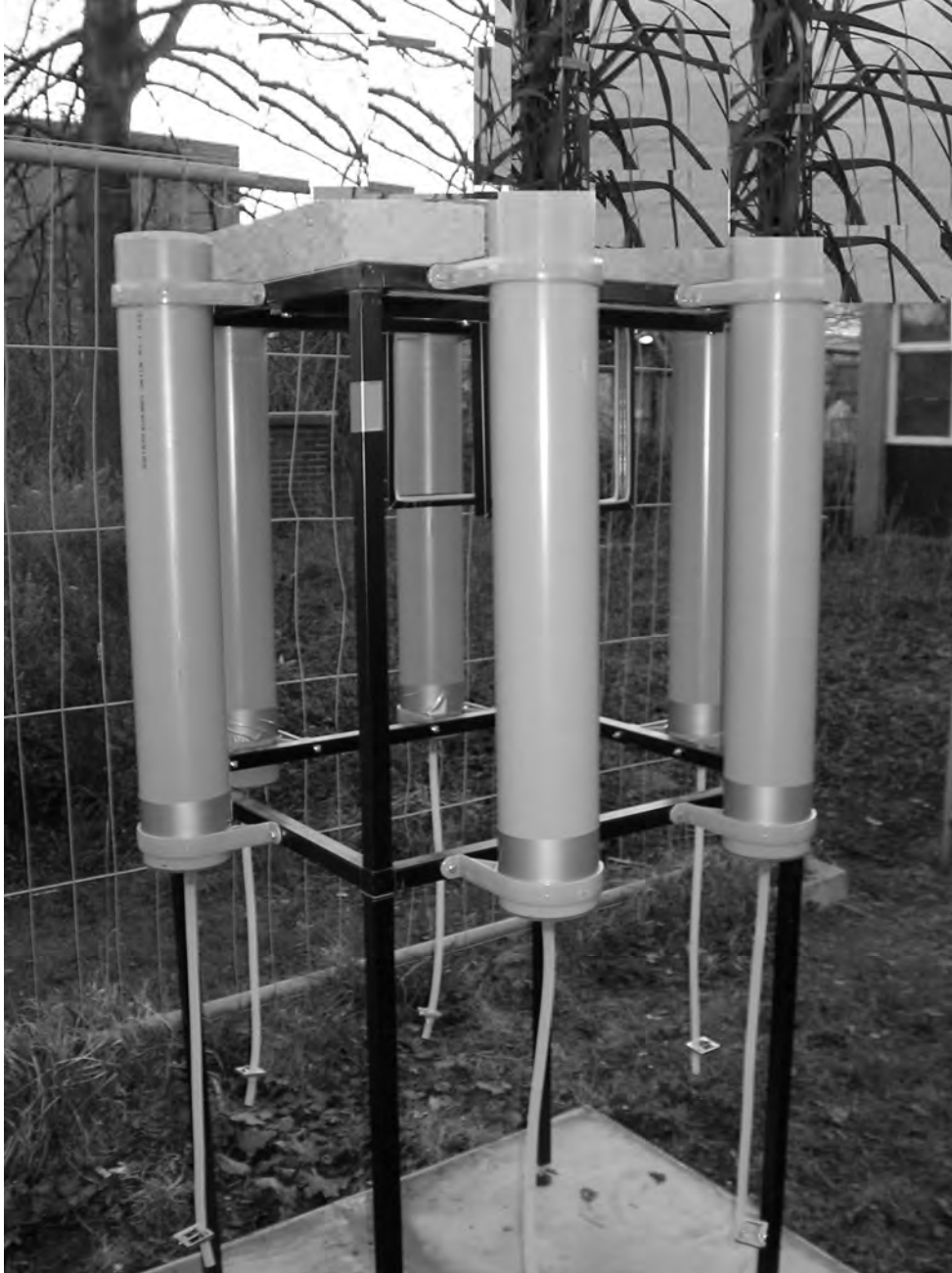
Figure 3-4. Experimental vertical-flow wetland rig located outside The King's Building's campus (June, 2006)
