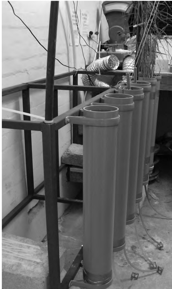
Figure 3-5. Experimental vertical-flow wetland rig located inside (Temperature, humidity and partly controlled room) on The King's Building's campus (a) fully controlled (June, 2006) (b) early control stage (October, 2005).
