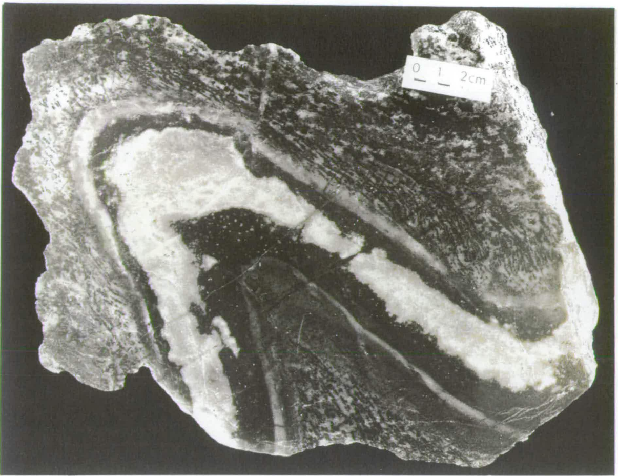
Figure 9.23 Small fold ( F_1 ) in calc-silicate layer from the Chelnok Paragneiss. Calc-silicate layer and early foliation (pre- S_1 ) have been folded and a new fabric developed axial planar to this fold ( S_1 ). This S_1 fabric is orientated 38^\circ to 350^\circ and the fold axis plunges at about 40^\circ to 020^\circ .
