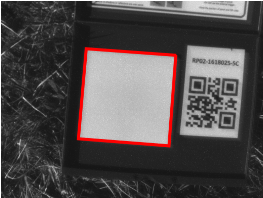
Figure 3-8 | Parrot Sequoia pre-flight radiometric calibration image of a MicaSense Ltd. (Seattle, WA, USA) reflectance target in the near-infrared band. Red box: surface with known reflectance value used for calibration.
