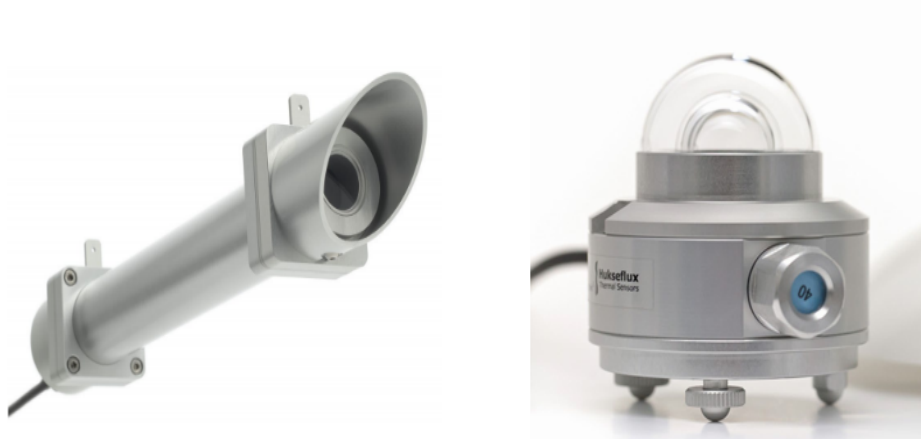
Figure 2.8 (Left) First class of pyrheliometer (right) First class of pyranometer [75]
