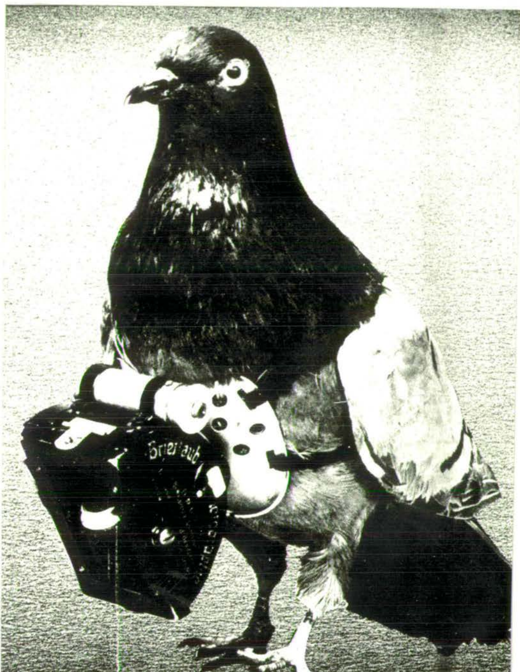
FRONTISPIECE: AN EARLY REMOTE SENSING PLATFORM The pigeon camera and its carrier-pigeon
