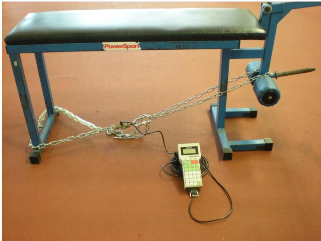
Figure 5.2: Bench equipment set up for isometric maximal voluntary contraction for both knee extension (using the illustrated strain gauge) and knee flexion.
