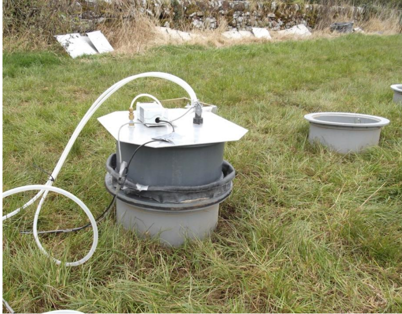
Figure 3.6 The dynamic chamber was placed on top of static chamber bases at the Dumfries field site to verify static chamber flux measurements. The rubber flap was rolled down prior to measurements to avoid wind penetration of the neoprene sponge seal.
