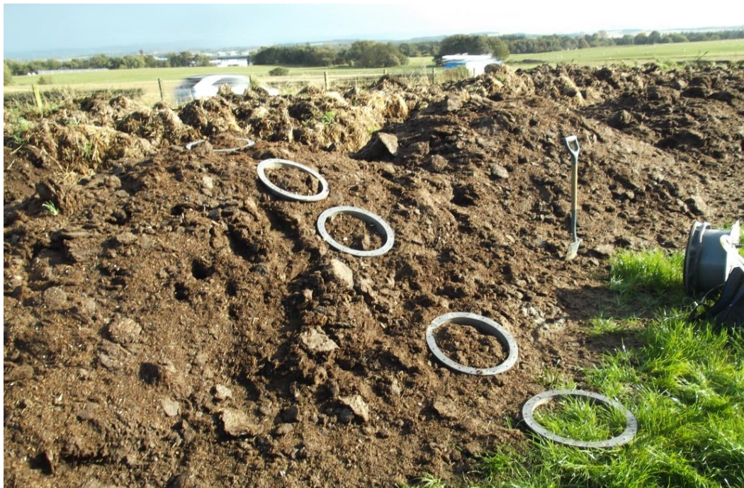
Figure 7.7 Dynamic chamber measurements were made from manure heaps from various fields during the farm scale experiment. The rings fit into the surface of the heap as they would on soils. Fluxes from silage grass and animal barns were measured in a similar way.
