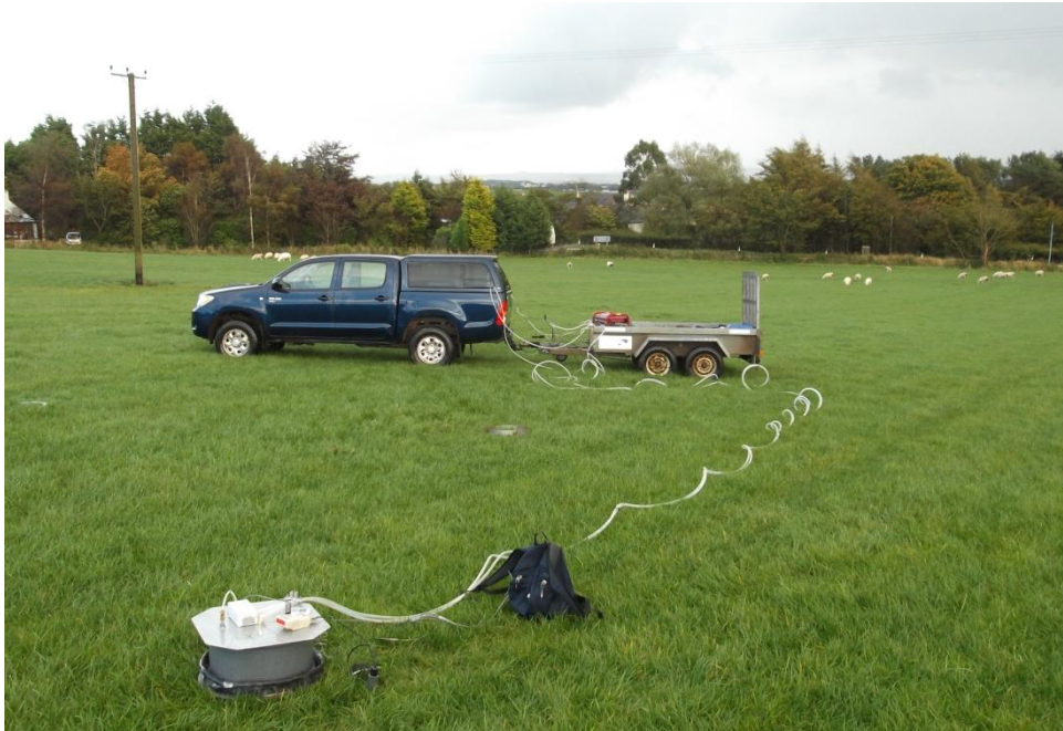
Figure 7.3 The QCL was mounted in an off road vehicle which was powered by a diesel generator. The dynamic chamber measurements could be made in a 30 m radius around the parked vehicle.
