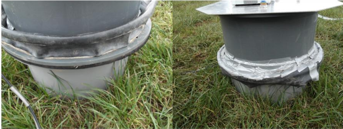
Figure 4.5 A skirt made from a rubber bicycle tyre was fitted to the chamber to prevent wind disrupting measurements. Prior to this, the neoprenes sponge fitted to the bottom of the chamber was expected to prevent a draught between the flanges between the chamber and base (left). The skirt was folded down across the connection between the chamber and chamber base to prevent leaks caused by high winds (right).
