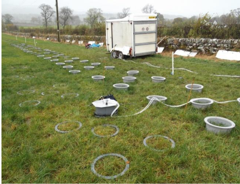
Figure 4.3 Measurements were made at the Dumfries field site set up and maintained by SRUC. Dynamic chamber measurements were made from consecutive plots of different fertiliser treatments from static chamber and cutting ring bases. The QCL was housed in a tow van and powered by a diesel generator at the site.
