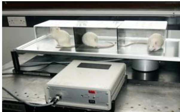
Figure 2.3. Photograph showing set up for Hargreaves' test to measure thermal hyperalgesia.
