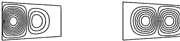
(b) a/b_1 = 1.5 , \beta = 0.8 . First and second buckling modes having buckling factor, k = 7.4968 and k = 8.8511 respectively.
