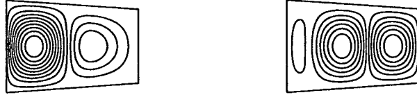
(a) a/b_1 = 1.4 , \beta = 0.8 . First and second buckling modes having buckling factor, k = 7.5452 and k = 8.8566 respectively.
