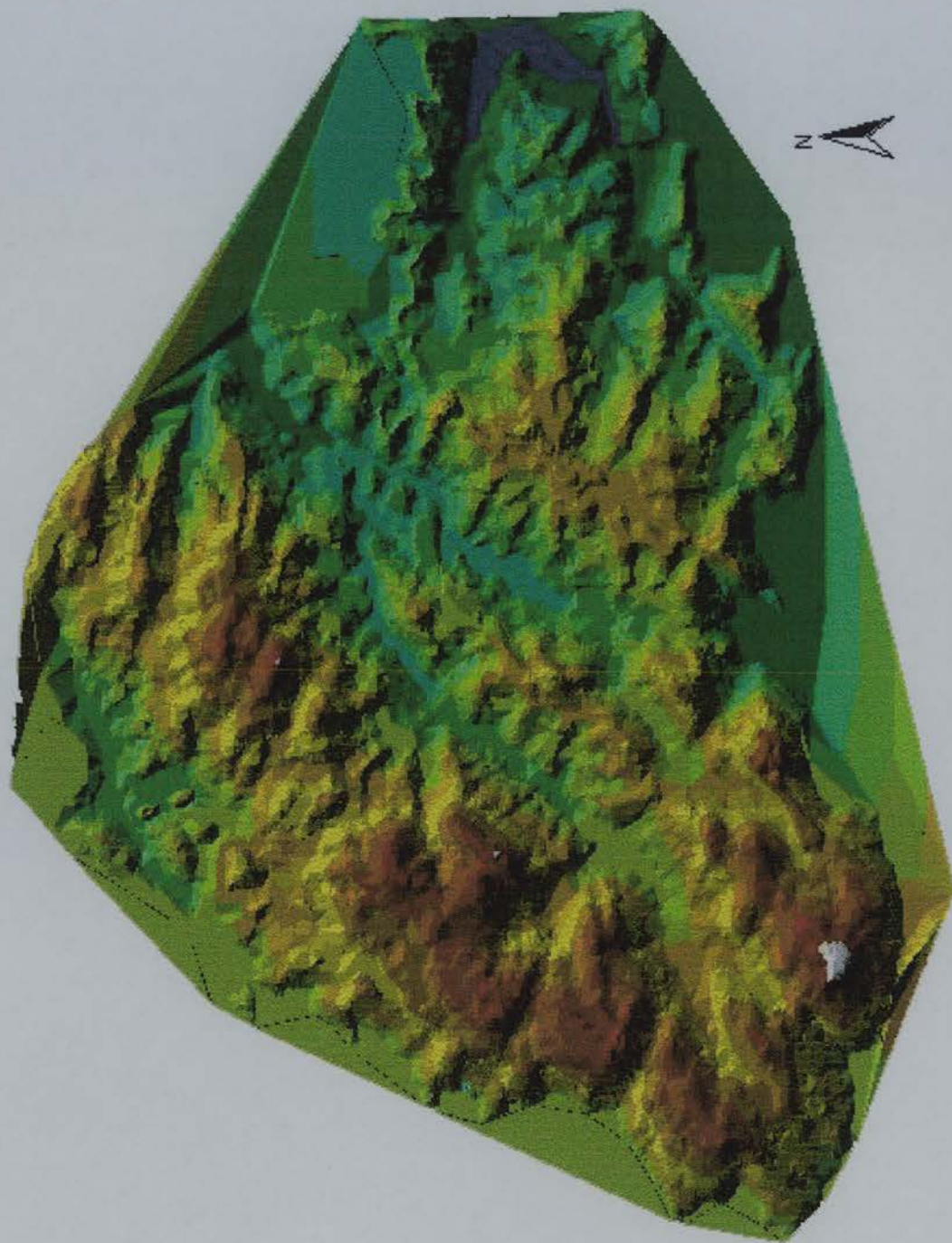
Figure 8.3. Hypsometric model of the Macaé de Cima terrain, derived from a TIN DTM (approximate scale 1:100,000). The colours represent eleven altitudinal levels (from 880m to > 1660m a.s.l., at 80m intervals).
