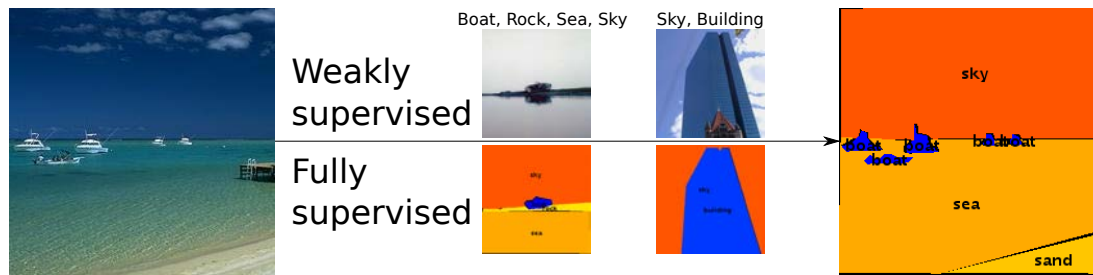
Figure 3.1: Semantic segmentation is the task of assigning class labels to all pixels in the image. During training, with full supervision we have ground-truth labels of all pixels. With weak supervision we only have labels at the image-level. For more information refer to Sec. 2.1.
