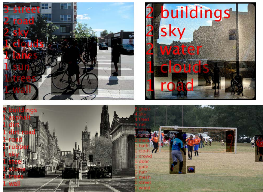
Figure 7.1: Image-level annotations overlaid on example images of the ImageNet-Stuff dataset. The images shown are selected to include instances of the car class. All known thing instances are masked with a black box. Together with the ground-truth image-level tags, we show the absolute frequency that indicates how many annotators used the same label or synonyms thereof.
