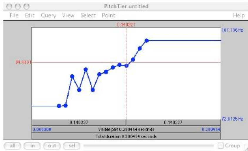
Figure 5.3: Praat pitch tier, from Cambell-Kibler (2006, p. 89). Pitches could be manipulated by dragging dots to desired pitch levels.
