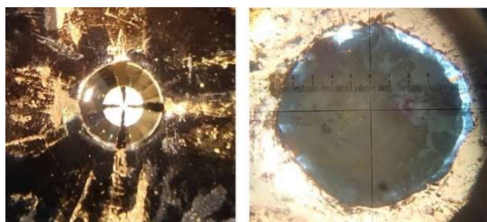
Figure 3.2 On the left: Diamond with gold sputtered contacts (no sample). On the right: IBN sample within a gasket hole under 5 GPa. The transparent light blue areas between inner gasket hole and sample represent PVC layer.
