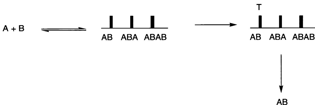
Scheme 3 Preequilibrated DCL: a DCL in generated by reversible reaction of A and B then frozen. The frozen library is then screened for activity against target T .
