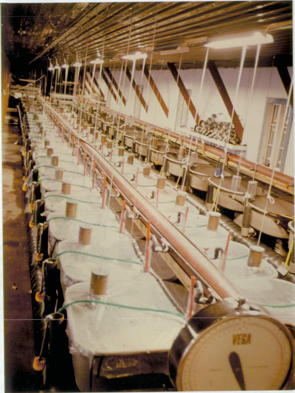
Figure 3.2. An overview of the experiment during the 1979/80 season. The central red pipe supplies inlet water. The water flow controllers are mounted adjacent to this pipe, one per tank. The green tubes carry overflow water from the controllers. The top halves of the automatic feeders are protruding from the plastic covers. Each tank's central drain leads to a black waste pipe, one pipe per row.
