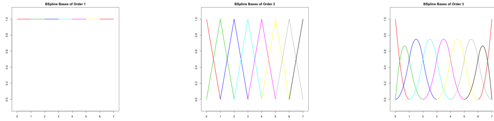
(a) Seven bases of order 1. (b) Eight bases of order 2 that are linear combinations of bases of order 1. (c) Nine bases of order 3 that are linear combinations of bases of order 2.
