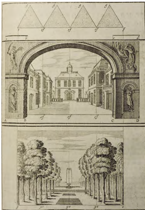
Fig. 1.4 Jean Dubreuil, La Perspective Pratique , 1649, Traité IV, Pratique 11. Combination stage system of periaktoi and flats.
