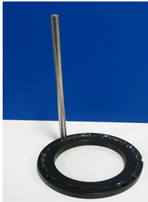
Figure 7.5 Membrane-ring-membrane (MRM) “sandwich” . A thin, acoustically transparent membrane was placed between two Derlin rings so as to form a compartment where cells could be grown.
