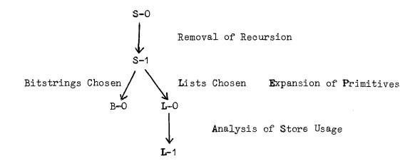
The steps S-O->S-1, S-1->B-O and S-1->L-O are the steps where the main flattening of the functional tree takes place.
