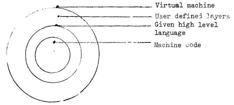
In our system L-1 or B-O is the given language, S-O the final virtual machine and S-1 and L-O the intermediate layers.
