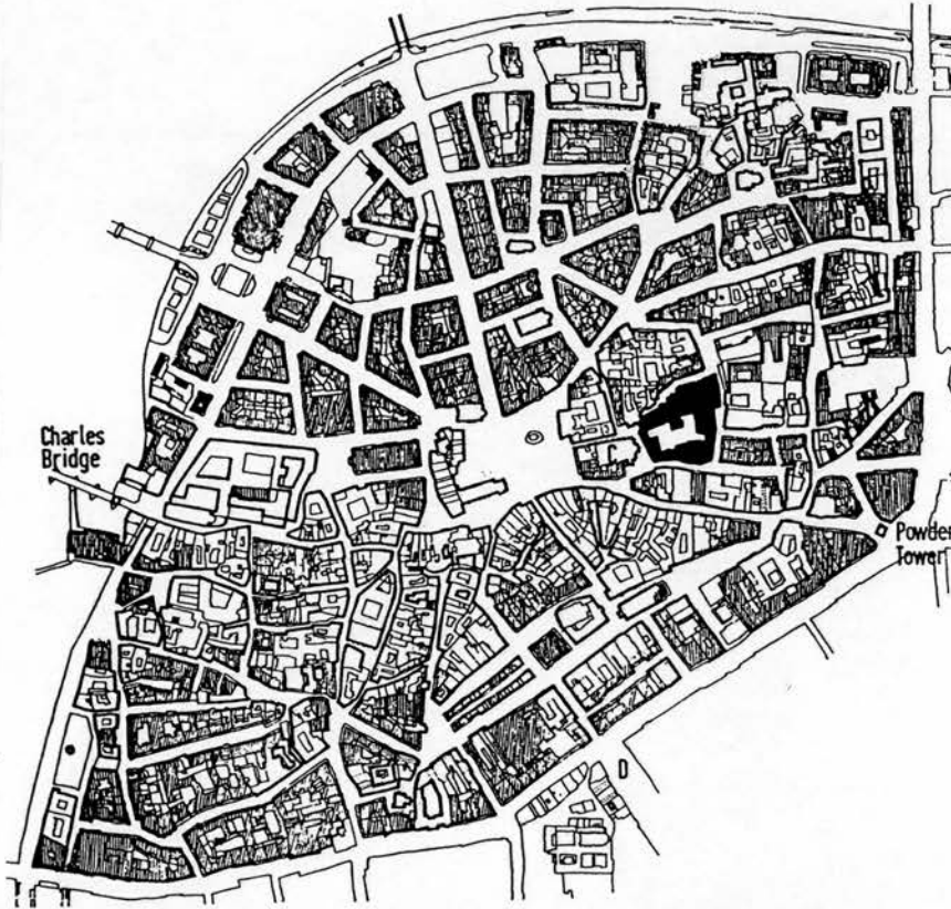
Figure 3.2: The old town of Prague; the defensive wall of 1235 was demolished in 1760 to form the line of east-bank inner-ring boulevard. Notice the similarity in the planning principles with the city of Arriyadh Figure 3.4, particularly in the southern sector where Renaissance planning has not over ridden the medieval street pattern.
