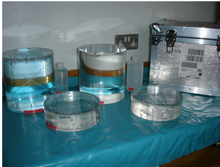
Figure 2.3: Standard Magnet Phantom set for baseline QA including a good old SNR/Uniformity phantom, a Geometric Linearity/Distortion and Slice Width phantom, a Spatial Resolution phantom, and a Slice Position phantom and a Copper Sulphate filled bottle phantom
