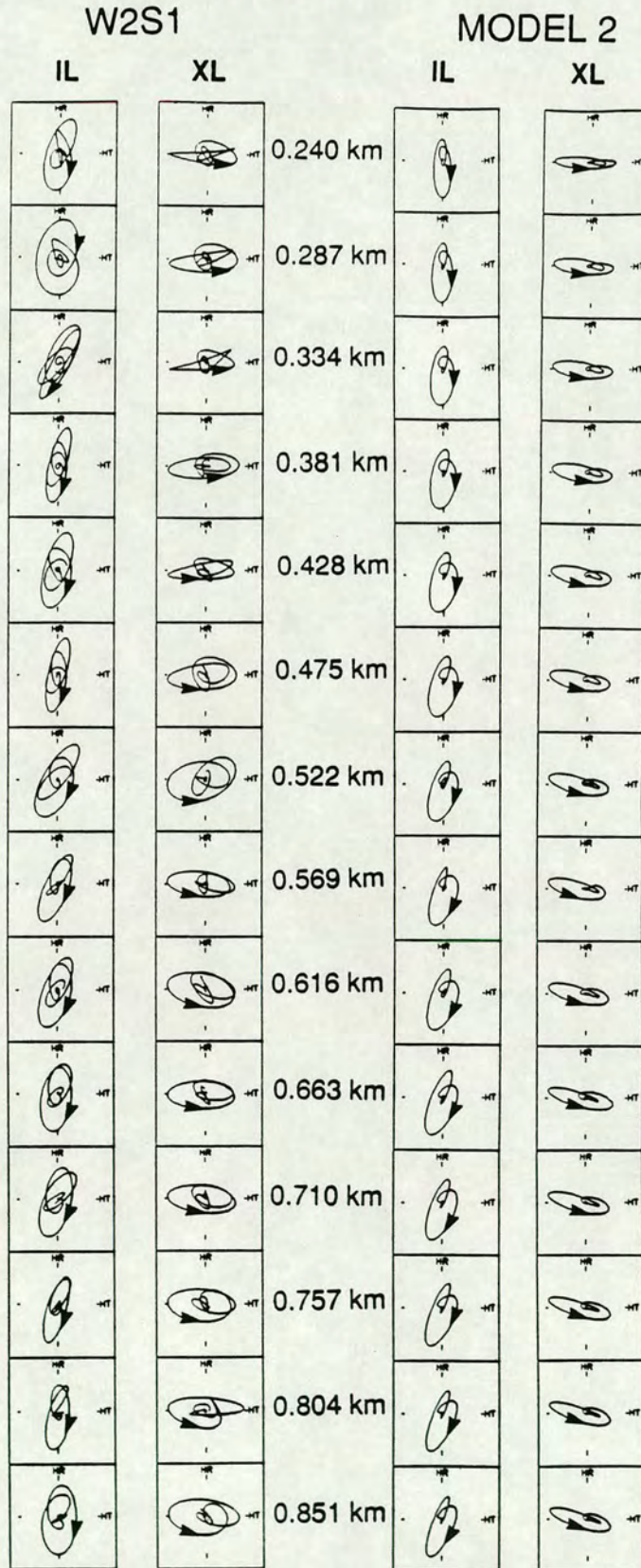
FIGURE 6.5: Selected observed and modelled horizontal plane shear-wave polarization diagrams from the 115m offset VSP for Model 2. The direction of motion is marked by an arrow.
