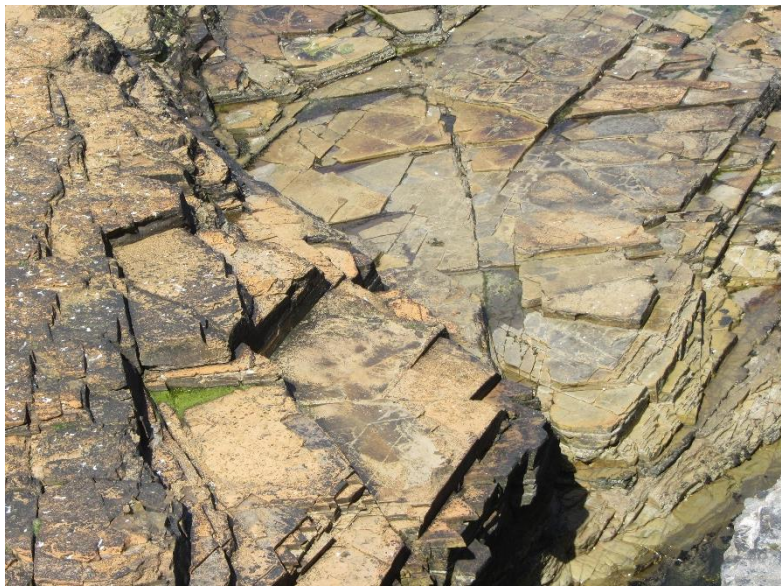
Figure 46 Typical Orcadian bedrock exposure of flagstone formation with (here) horizontal bedding planes and vertical cleavage planes at 30, 60 and 90 degrees to each other. This produces first class building stones with minimal quarrying cost.
