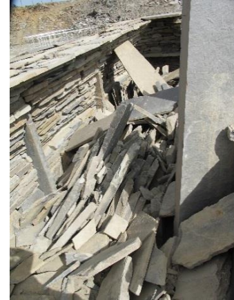
Figure 126 (right) Cascade of corbel slabs experimentally built and forced into failure at Spittal Quarry experimental centre 2006
