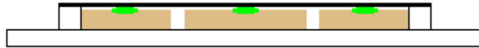
Figure 3.3: Schematic of sample chamber used in experiments. Bacterial samples (green), are pipetted onto three agarose pads (brown), held in place by a microscope slide (bottom), GeneFrame, (sides), and sealed with a coverslip (top). The entire sample is then inverted and imaged using the confocal microscope.
