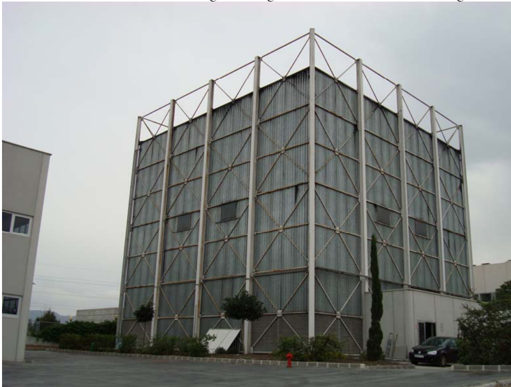
Figure 1. Photo of the 20 m high atrium facility used in the Murcia Atrium Fire Tests, Murcia, Spain.
